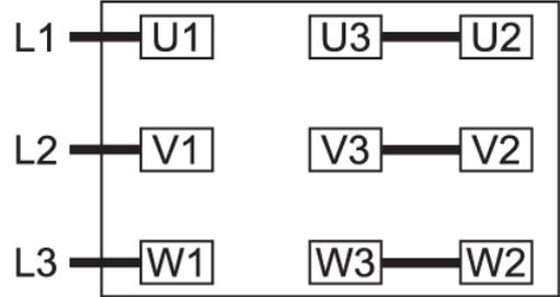
Double star connection, multi-voltage motor with 12 pins (low voltage):
