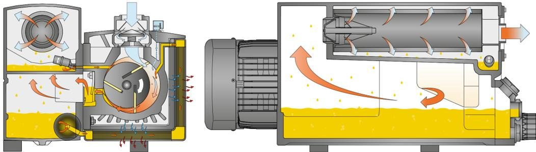
The machine works on the rotary vane principle.
