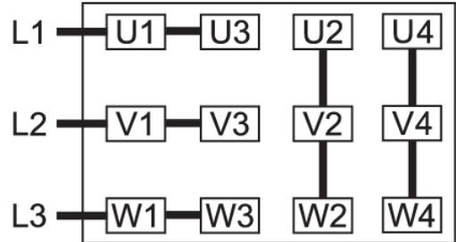
Star connection, multi-voltage motor with 12 pins (high voltage):
