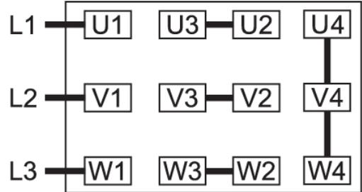
Delta connection, multi-voltage motor with 12 pins (middle voltage):
