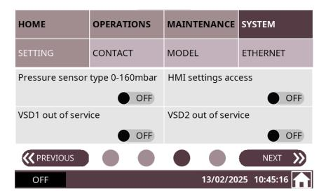
On the third screen/page, it is possible to access the internal settings of the HMI by pressing the button for two seconds.
