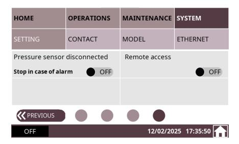
On the fourth screen/page, if a pressure sensor is installed, it is possible to activate/deactivate the **pressure sensor disconnection** alarm.
