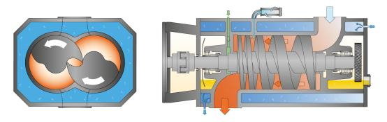
The machine works on a two-stage twin-screw pump principle.
