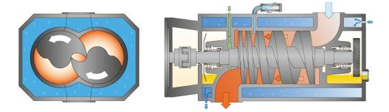
The machine works on the one-stage, twin-screw pump principle.
