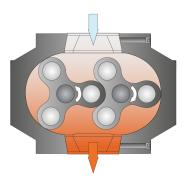
The machine with tri-lobe rotors works on the principle of oil-free gas transport.
