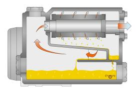
The machine works on the rotary vane principle.
