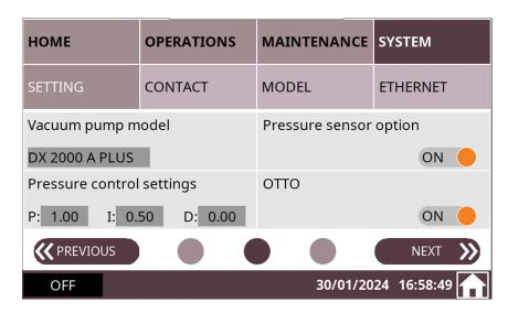
On the second screen/page, it is possible to edit some pump parameters like the pressure control settings (PID) or to activate/deactivate pump functions like the pressure sensor (Option) or OTTO.
