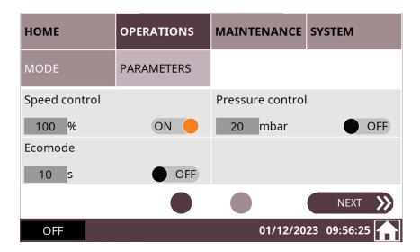
Speed control (Standard). Configured by default with a vacuum pump speed of 100 %, the speed control mode allows the variation of the motor frequency.
