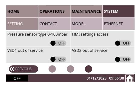
On the third screen/page, if a pressure sensor is installed, a 0 ... 160 mbar range is displayed:
