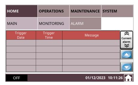
When an alarm occurs, an audible alarm sounds, and the user must acknowledge the default on the HMI interface.
