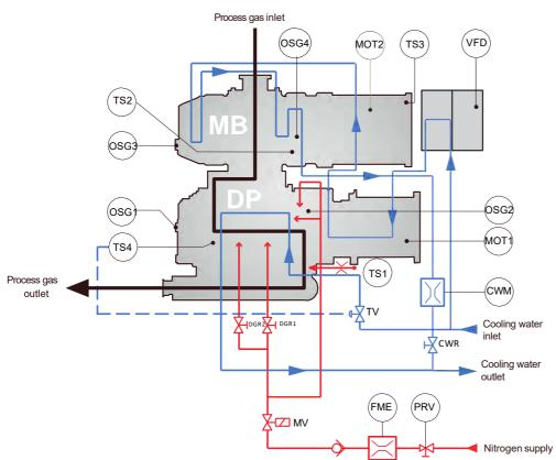
FME Nitrogen flow meter, dilution gas
