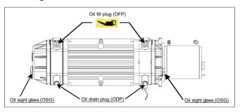
NOTE: The quantity of oil specified in the installation handbook is of informative nature only. Check the oil level with the help of the various oil sight glasses (OSG) on the vacuum pump.
