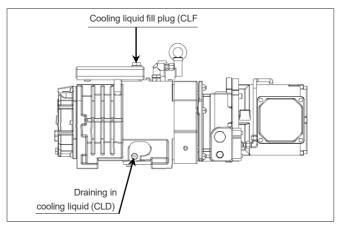
DS 1800 A H Installation and Commissioning 0870741408 (EN) **NOTE**: The quantity of cooling liquid specified in the installation handbook is of informative nature only. Respect the procedure of filling the cooling liquid.
