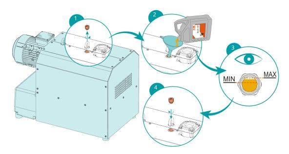
The oil level should stay constant over the lifetime of the oil. If the level does fall, this indicates a leak and the machine requires repair.
