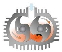
The machine works on the claw principle.
