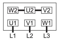
Double star connection, multi-voltage motor with 9 pins (low voltage):
