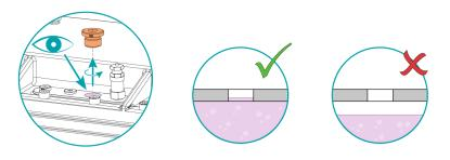
• Fill up if necessary, see Filling Cooling Liquid [ $\rightarrow$  19].
