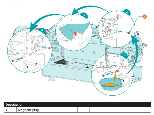
For oil type and oil capacity see Technical Data and *Oil* [ $\rightarrow$  45].
