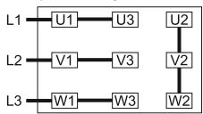
Double star connection, multi-voltage motor with 12 pins (low voltage):
