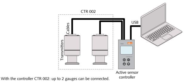
• Connect the cable from the controller to the gauge.
