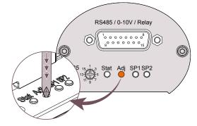
• Remove the rubber cap above the "Adj" pushbutton.
