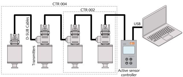
With the controller CTR 002: up to 2 gauges can be connected. With the controller CTR 004: up to 4 gauges can be connected.
