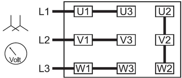
Star connection, multi-voltage motor with 9 terminals (high voltage):
