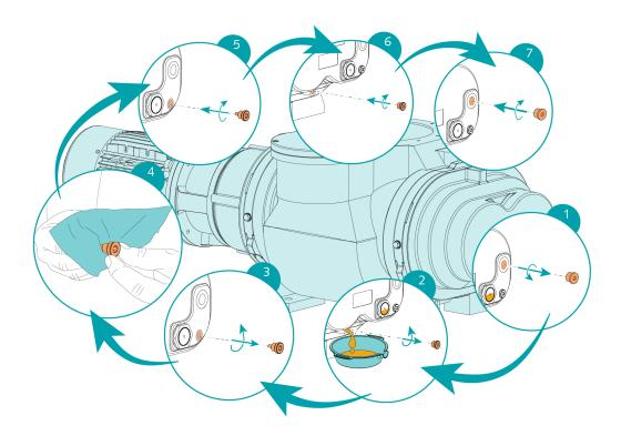
For oil type and oil capacity see *Technical Data* [ $\rightarrow$  29] and *Oil* [ $\rightarrow$  30].
