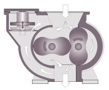
The machine works on the Roots blower principle.
