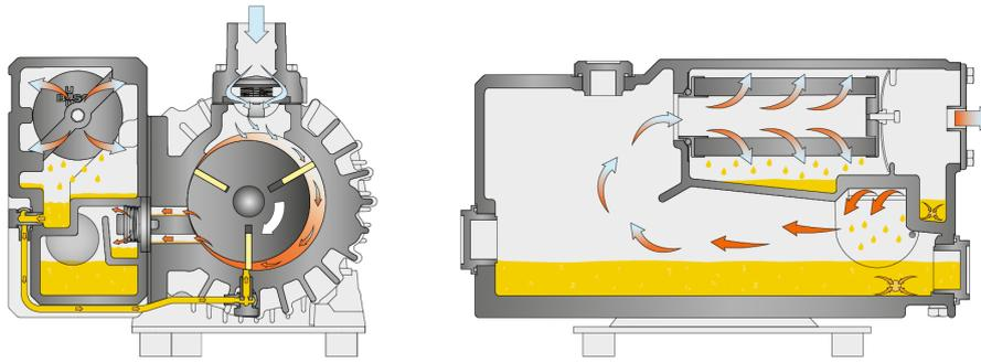
The machine works on the rotary vane principle.
