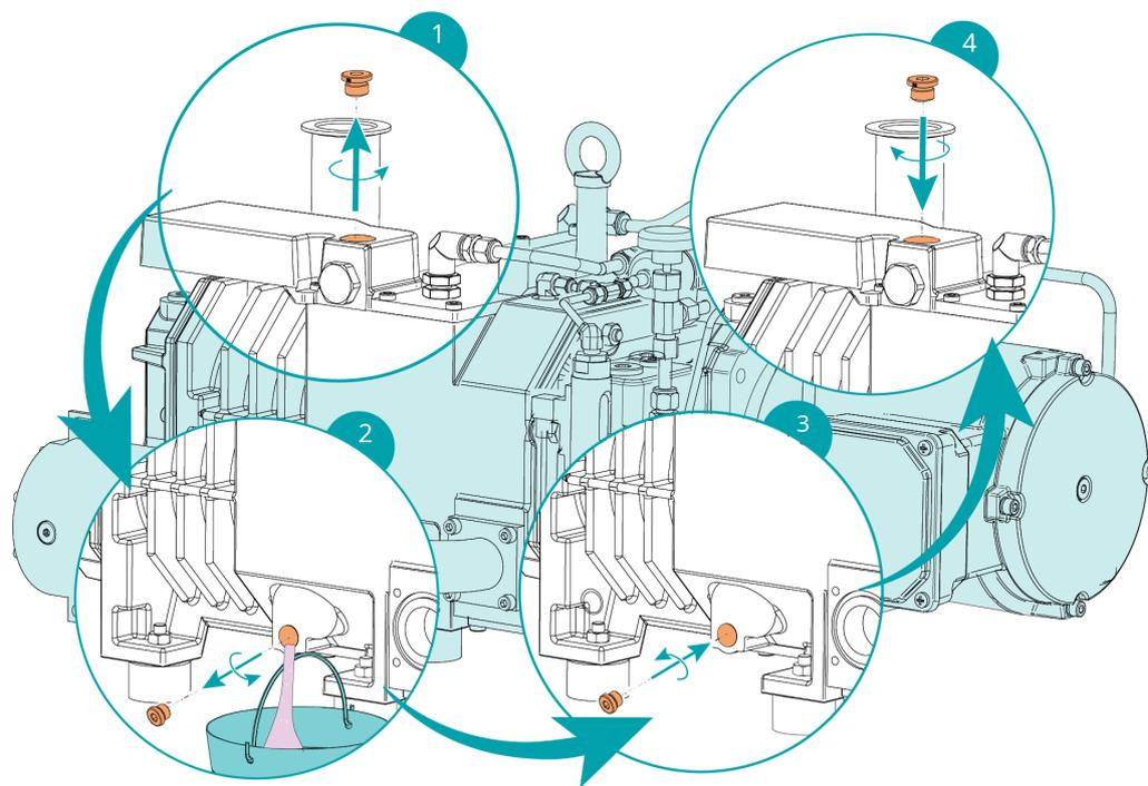
For cooling liquid type and cooling liquid capacity see Technical Data and *Cooling Liquid* [→ 39].
