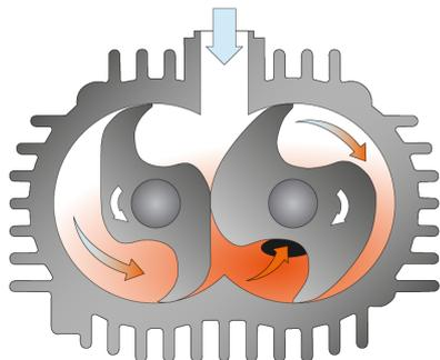
The machine works on the claw principle.
