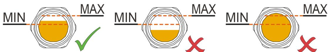
The oil level should stay constant over the lifetime of the oil. If the level does fall, this indicates a leak and the machine requires repair.
