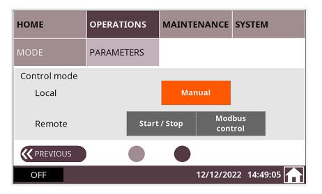
The second screen/page of the display "OPERATIONS > MODE" shows the **Control mode** of the machine (**Local** > **Manual** or **Remote** > **Start/Stop** or **Modbus control**).
