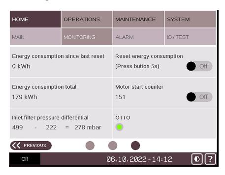
**Energy consumption since last reset:** Indicates the energy consumption in kWh since the last reset.
