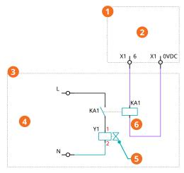
Inlet Valve Wiring Diagram
