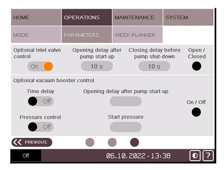
The system allows a time delay between the opening of the valve and the start-up of the vacuum pump (Default value 10s).
