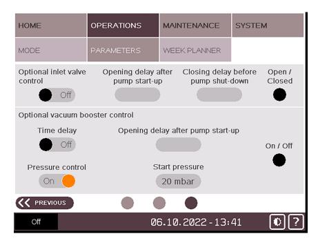
The booster start signal is given by the PLUS pump when the pressure reaches a set value (Default value 20 mbar).
