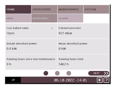
Gas-ballast valve: Indicates the state of the gas ballast valve ▶ "Open" or "Closed", see Gas Ballast *Valve Control*  $[\rightarrow 43]$ .
