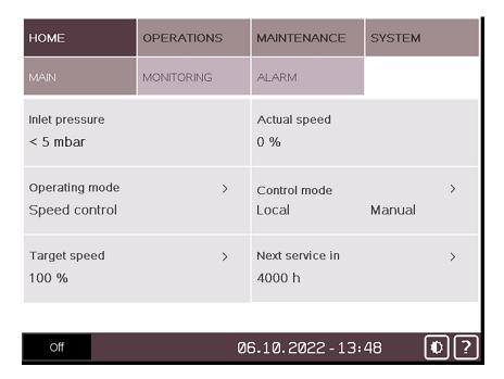
**Inlet pressure:** Indicates the operating pressure at the suction connection (IN) according to the selected unit. To change the unit, see *System Settings*  $[\rightarrow 13]$ .
