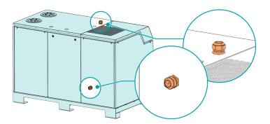
Electrically connect the control unit to the power supply and connect the protective earth connection according to the electrical scheme, see Wiring Diagram Control Unit [→ 33].
