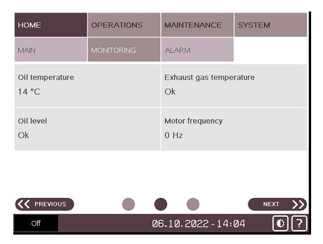
**Oil temperature:** Indicates the oil temperature, in case of a too high temperature a warning or an alarm occurs, see *Dysfunction* [ $\rightarrow$  55].
