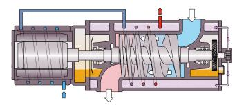
The machine works on the one-stage, twin-screw pump principle.
