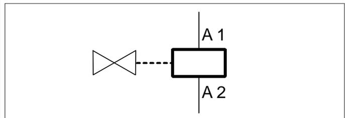
**Pressure switch connection on the seal fluid separator**
