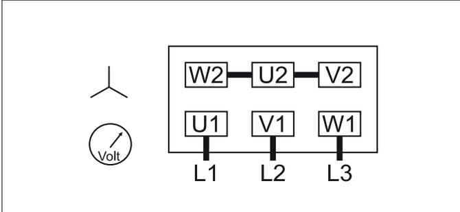
Star-star connection, multi-voltage motor (Low voltage)
