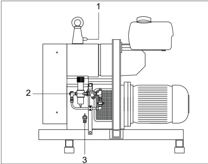
Direct cooling with temperature regulating valve
