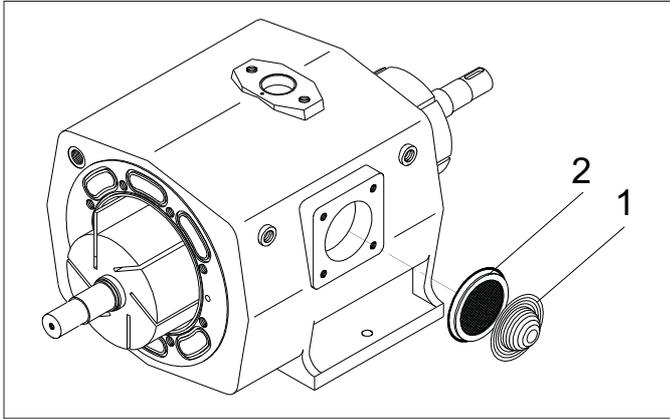
These screens must be assembled before the suction inlet. They prevent dirt particles from entering into the vacuum pump.
