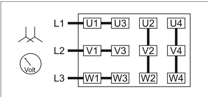
Delta connection, multi-voltage motor (Middle voltage)
