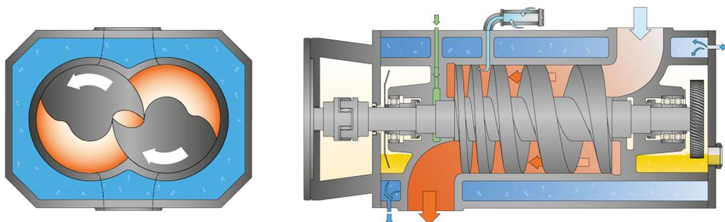
The machine works on a two-stage twin-screw pump principle.
