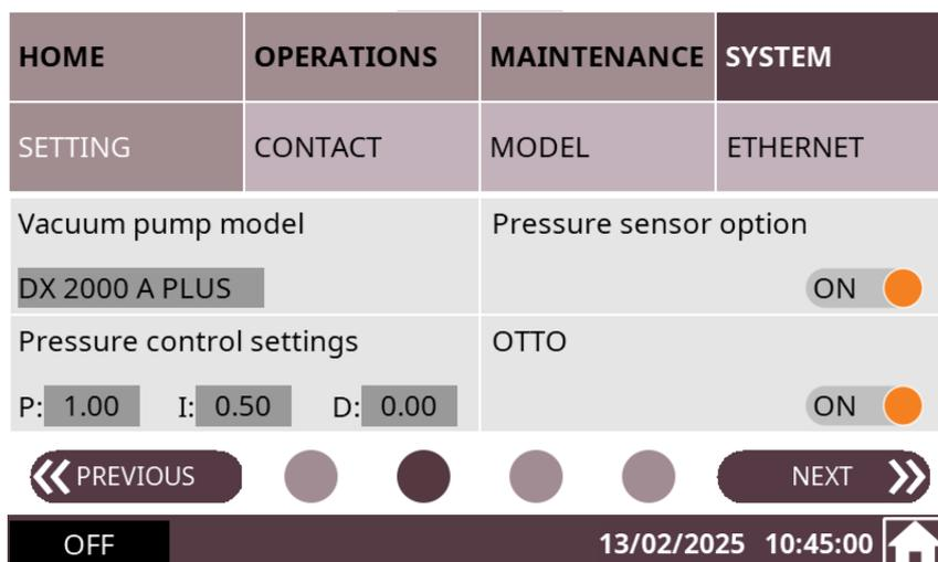
On the second screen/page, it is possible to edit some pump parameters like the pressure control settings (PID) or to activate/deactivate pump functions such as the pressure sensor (Option) or OTTO.
