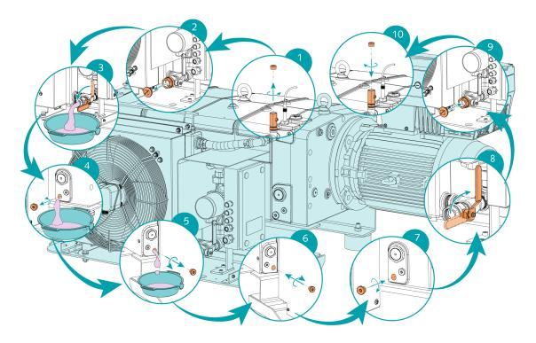
For cooling liquid type and cooling liquid capacity see Technical Data and *Cooling Liquid* [→ 46].
