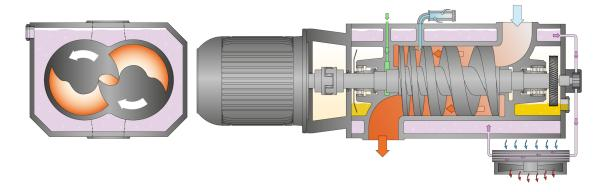
The machine works on the one-stage, twin-screw pump principle.
