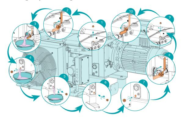
For cooling liquid type and cooling liquid capacity see Technical Data and *Cooling Liquid* [→ 44].
