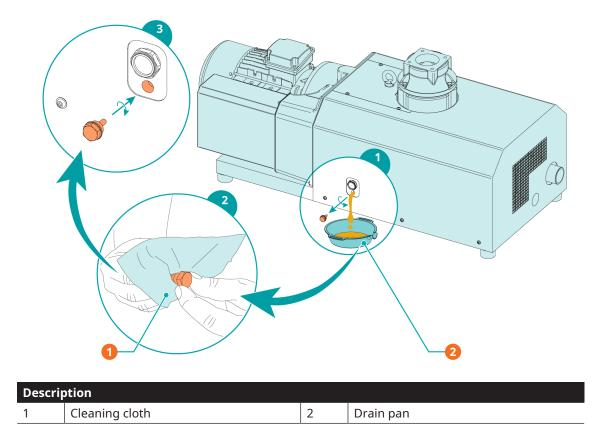
For oil type and oil capacity see *Technical Data* [ $\rightarrow$  29] and *Oil* [ $\rightarrow$  30].
