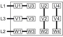
Delta connection, multi-voltage motor with 12 pins (middle voltage):
