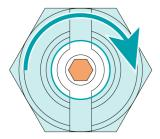
• Adjust the relief valve position by closing the valve (increase the spring resistance) by a counter-clockwise rotation to achieve 450 hPa (mbar) absolute +/- 5 hPa.
