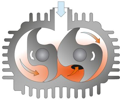
The machine works on the claw principle.
