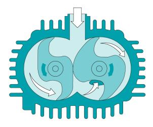
The machine works on the claw principle. The MINK is fully air-cooled.
