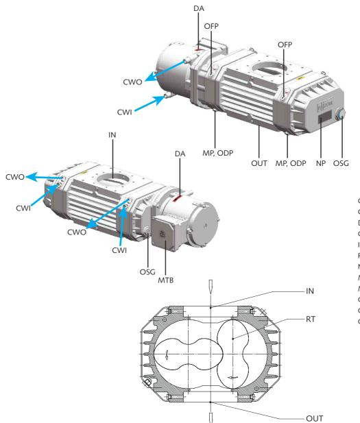
CWI Cooling water inlet CWO Cooling water outlet DA Directional arrow OFP Oil filler plug IN Inlet RT Rotor NP Nameplate MP Magnetic plug MTB Motor electrical box ODP Oil drain plug OSG Oil sight glass OUT Outlet
