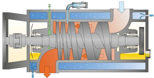
The machine works on a two-stage twin-screw pump principle.
