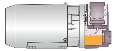
The machine works on the rotary vane principle.
