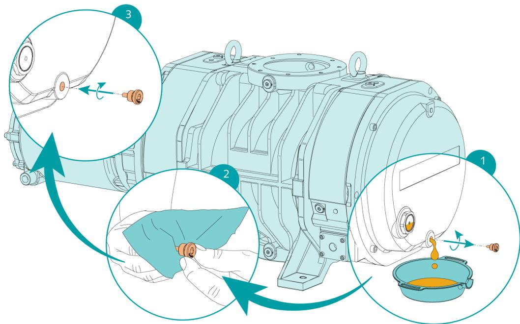
For oil type and oil capacity see *Technical Data* [→ 33] and *Oil* [→ 35] chapters.
