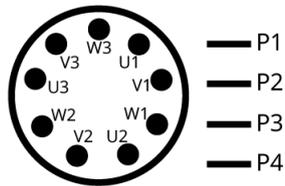
Connection of motor temperature switches (recommended):
