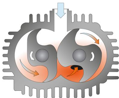
The machine works on the claw principle.
