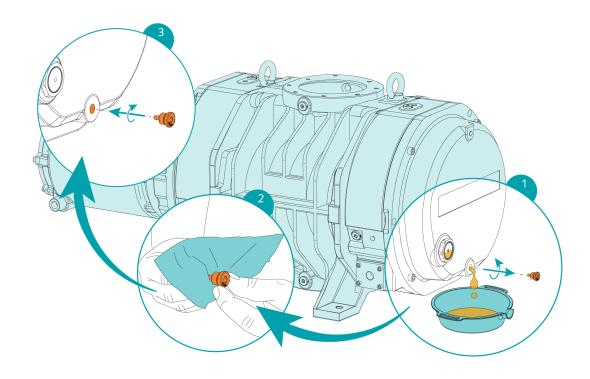
For oil type and oil capacity see *Technical Data* [ $\rightarrow$  30] and *Oil* [ $\rightarrow$  32].
