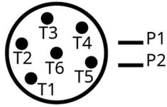
Connection of motor temperature switches (recommended):
