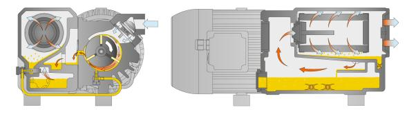
The machine works on the rotary vane principle.
