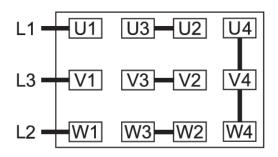
Delta connection, multi-voltage motor with 12 pins (middle voltage):
