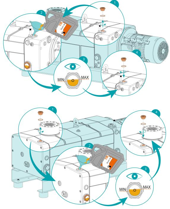
For oil type and oil capacity see Technical Data and *Oil* [ $\rightarrow$  37].
