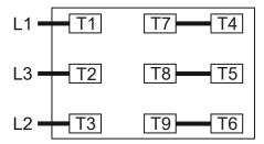
Connection of motor thermistors (3xPTC) (recommended):
