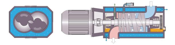
The machine works on the one-stage, twin-screw pump principle.
