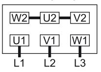
Star connection, multi-voltage motor with 12 pins (high voltage):
