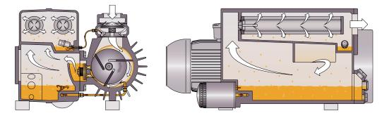
The machine works on the rotary vane principle. The oil seals the gaps, lubricates the vanes and takes away compression heat. The oil filter cleans the circulating oil. Exhaust filters separate the oil from the discharged gas.
