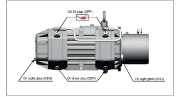
**NOTE:** The quantity of oil specified in the installation handbook is of informative nature only. Check the oil level with the help of the various oil sight glasses (OSG 1, 2, 3) on the vacuum pump.
