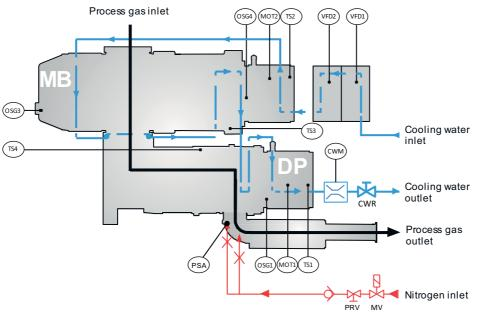
PRV Nitrogen pressure reducer PSA Pressure sensor TS 3 Oil temperature sensor (MB) (klixon) TS 4 Sensor PT100 OSG 1 Oil level indicator (DP) OSG 3 Oil level indicator (MB) OSG 4 Oil level indicator (MB) OFP Oil fill plug ODP Oil drain plug MOT 1 Motor (DP) MOT 2 Motor (MB) CWM Cooling water flow meter VFD 1 Frequency inverter (DP) VFD 2 Frequency inverter (MB) CWR Cooling water regulating valve MV Nitrogen solenoid valve TS 1 Klixon (DP) TS 2 Klixon (MB)
