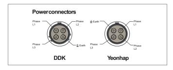
Connect the main cable on the socket, according to the following figure
