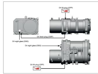
Oil filling on vacuum pump WY 0700 C
