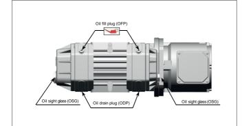
**NOTE:** The quantity of oil specified in the installation handbook is of informative nature only. Check the oil level with the help of the various oil sight glasses (OSG) on the vacuum pump.
