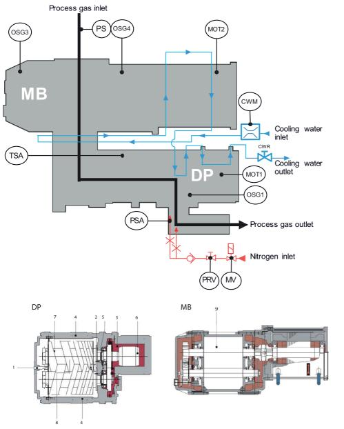
TSA Temperature sensor PRV Nitrogen pressure reducer PS Inlet pressure switch MV Nitrogen solenoid valve PSA Outlet pressure sensor OSG 1 Oil level indicator (DP) OSG 3 Oil level indicator (MB) MOT 1 Motor (DP) MOT 2 Motor (MB) CWR Cooling water regulating valve
