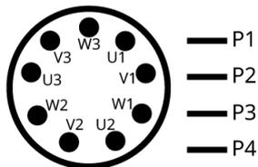
Connection of motor temperature switches (recommended):
