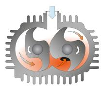
The machine works on the claw principle.
