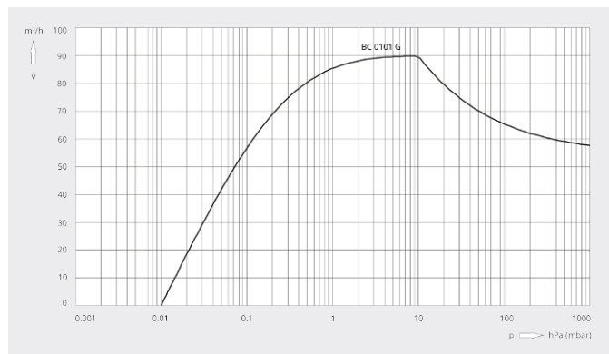
Pumping speed Air at 20°C. Tolerance: \pm 10\%
