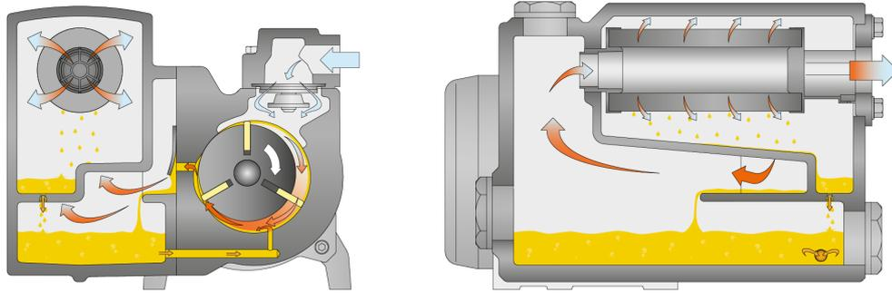
The machine works on the rotary vane principle.
