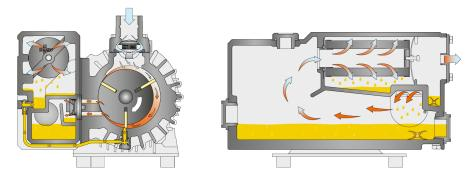
The machine works on the rotary vane principle.
